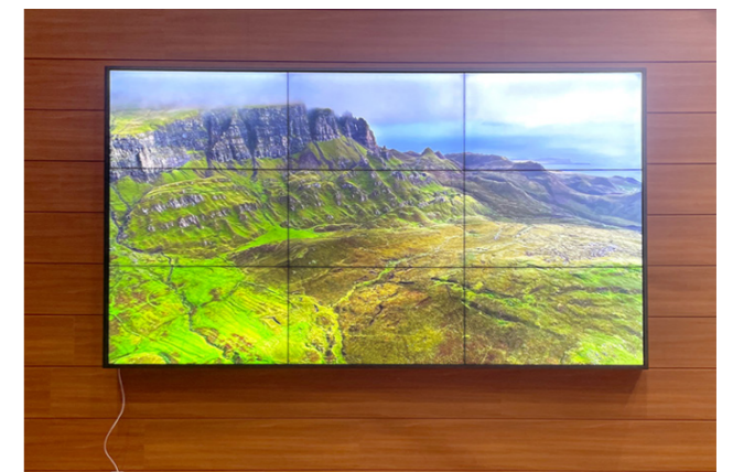
Dong A Health University Model: SYS-MWH-55E7A Specifications: 55Inch / 3x3 / Bezel 1.8mm / 700 nit
