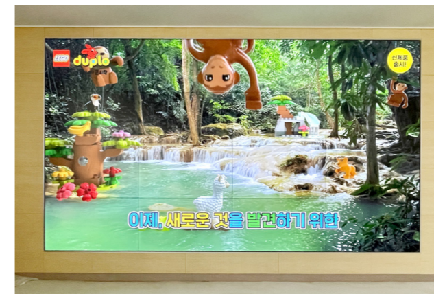
Hwasun Office of Education, Jeollanamdo Model: SYS-RNB-5502 Specifications: 55Inch / 4x4 / Bezel 0.88mm / 500 nit
