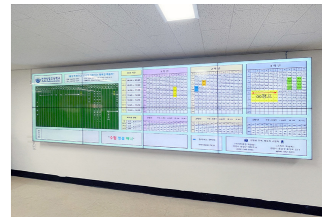
Cheonan Commercial High School Model: SYS-MWH-55E5A Specifications: 55Inch / 2x4 / Bezel 1.8mm / 500 nit
